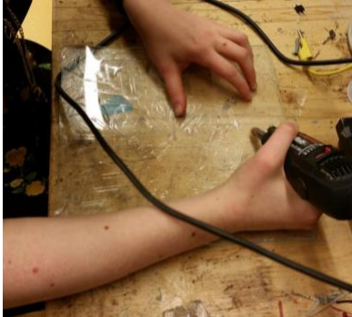
Figure 8: Dremeling the snowflake engravings by hand.
