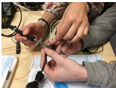
Figure 14: Soldering headers to wire endings for a modular easy-to-set-up design.
