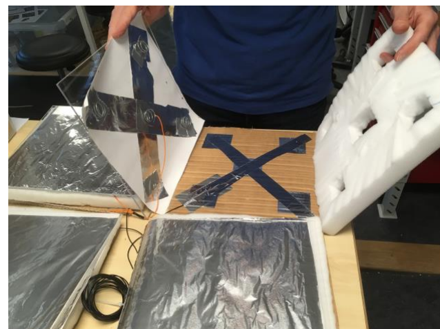
Figure 16: Tiles consisted of layers of cardboard, foam, conductive aluminium, and plexiglass.
