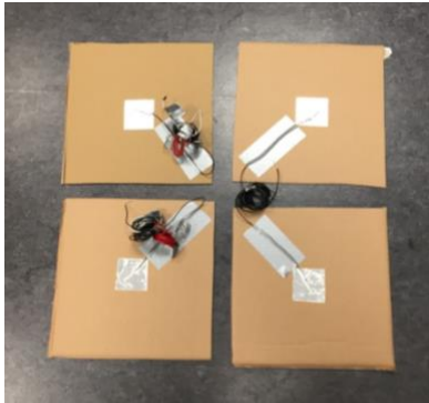
Figure 5: The bottom layer of the tiles is made of cardboard.
